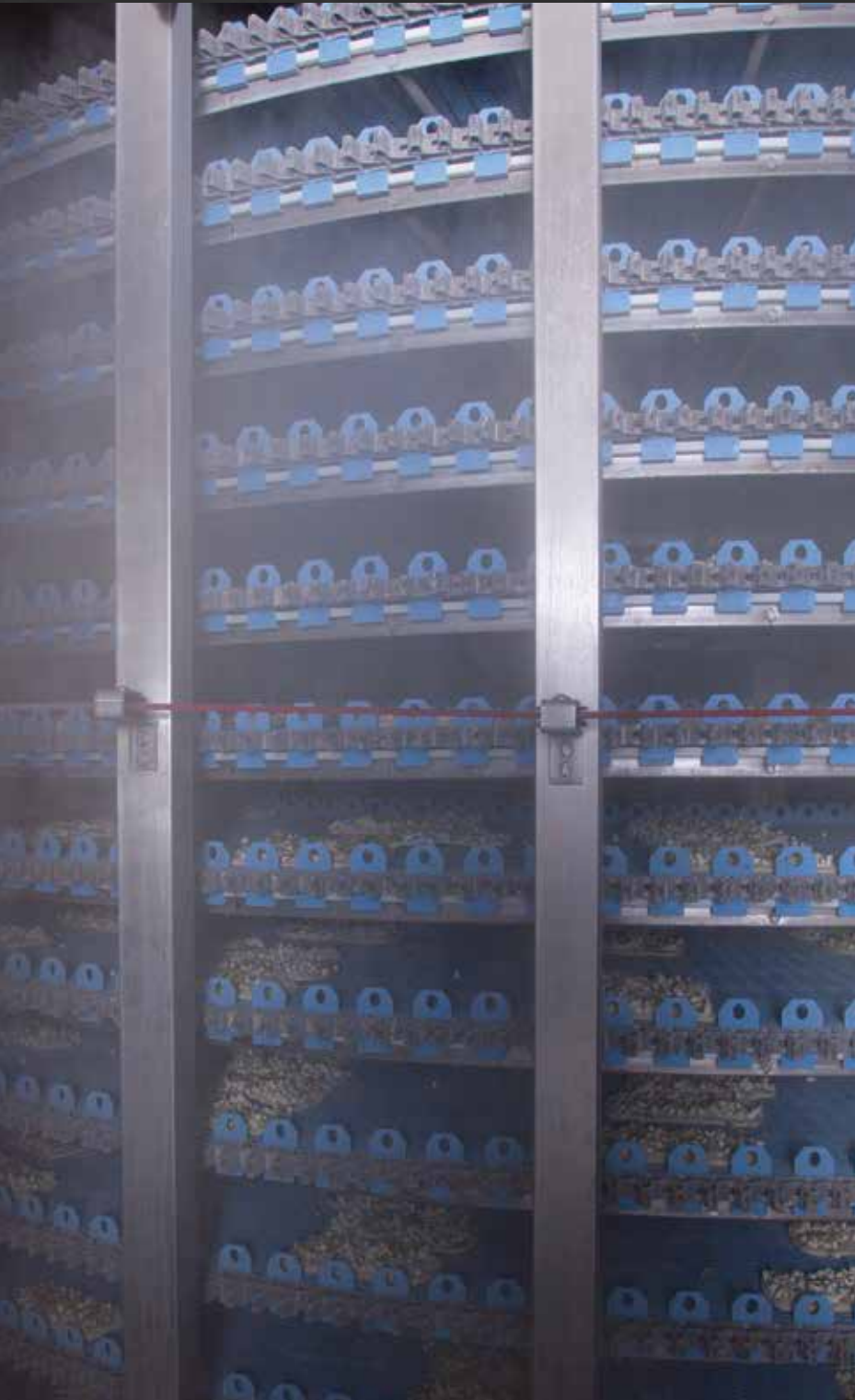
Flammkuchen slides in our fully automated blast freezer.
